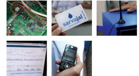
**ELECTRONIC/SENSOR BACKEND:** A basic input/output chipset equipped with LED display, RFID reader, and a basic telecommunication setup with a SIM card for each ATM.
